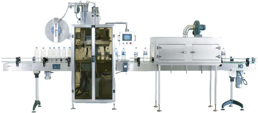
PVC Automatic Sleeve Shrink Labeling machine
